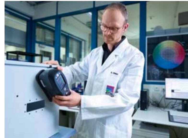
Laboratory-tested quality – Sebastian Otten checks whether enclosures are suitable for use in extreme offshore conditions at the accredited Rittal QA laboratory in Herborn. Here he is carrying out a test in the chemical-physical testing room, where a colour measurement is being performed on an enclosure surface.
