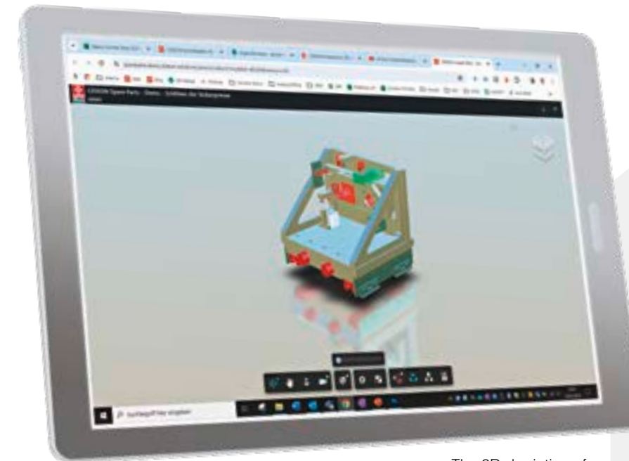
The 3D depiction of machinery and products in the spare parts viewer makes it easier to select the spare parts required.
