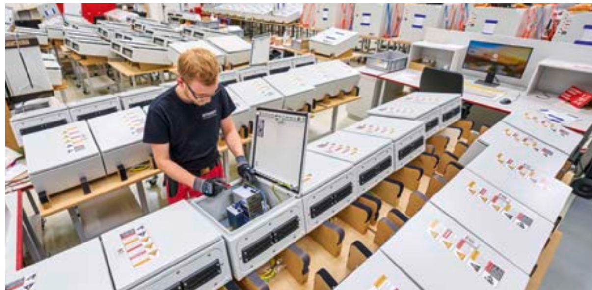
Beckhoff uses both KX enclosures (above) and AX compact enclosures from Rittal for the series production of its systems.
